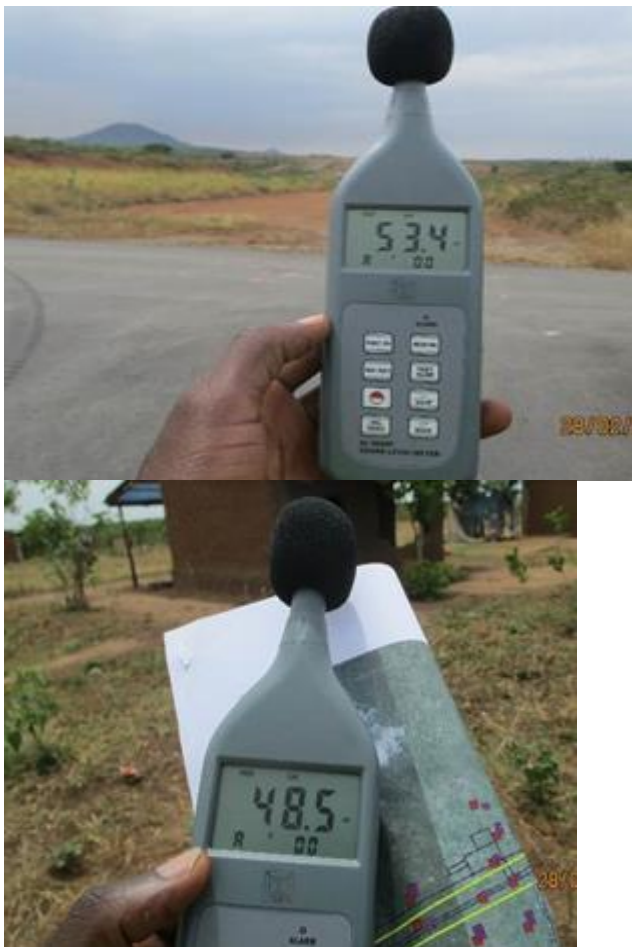
Figure 4.4: Noise Monitoring at the Kabaale Airport Construction area Source: SBC Environmental Report (2020)
